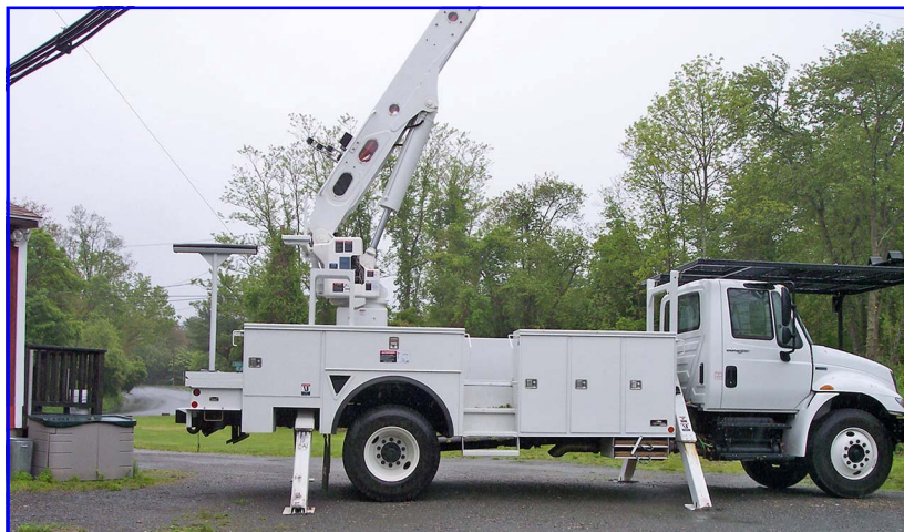
BUCKET TRUCK - JUST WHAT IS NEEDED TO WORK ON ANTENNAS!
