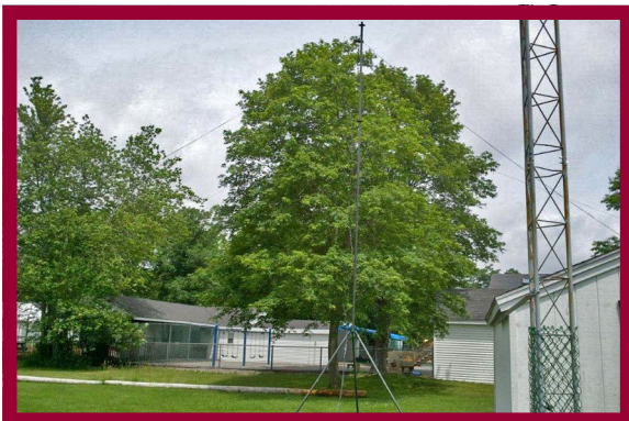
Center mast for the G5RV inverted vee
